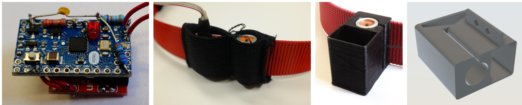
Figure 3.3: Arduino Mini and amplifier board, such an embedded synthesis unit together with a Haptuator in the initial belt pouch, and two subsequent iterations of the belt attachment.
