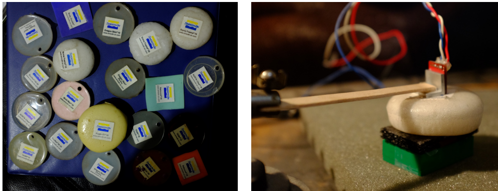
Figure B.5: One group of material samples, and an example accelerometer arrangement.
